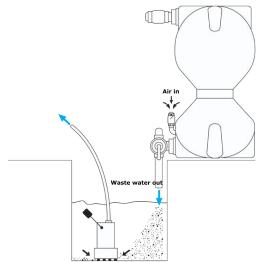
You can also connect a waste water pump directly to the filter waste outlet. In this situation, the filter can be installed below water level.
