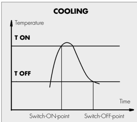
**NOTE:** When after setting the ON-OFF-temperature (heating) the actual temperature is within the temperature range (e.g. the relay is set to switch on below 20°C and switch off at 25°C and the actual temperature is 23°C), the relay will not switch. The relay will not switch on until the temperature falls below 20°C and off when reaching 25°C. The same principle applies for cooling actions.
